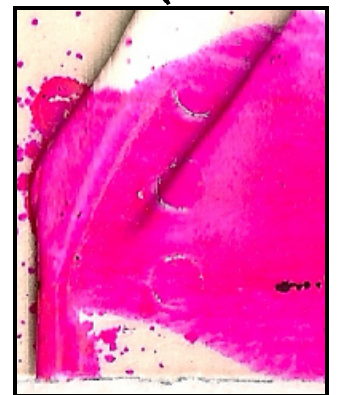
Figure 5. Faint holes at crease.
