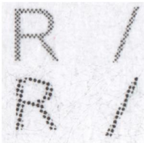
Figure 3 - Genuine APU "R" (top) and Counterfeit "R" (bottom)
